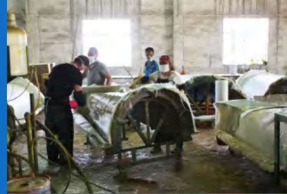
3-Laying fiber on mould
